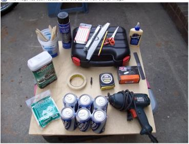
I used a 2'x2' piece of 5/8" particle board from Lowe's because it was cheap and is plenty strong enough for a low powered 8 in a box with no large flat surfaces. That one sheet wasn't quite enough, but I had some scraps laying around.
