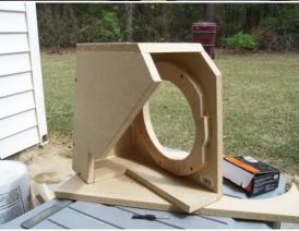
Now, on the last version I built I rushed the fiberglass work and it sagged inwards and too up valuable mounting depth, I couldn't flush mount. So this time I put a little Press-and-seal on the sub and installed it, so even if the cardboard does sag it can't take up the subs space. My other problem last time was using corregated cardboard. It's so thick once glassed that I might as well used wood and saved time.
