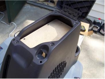
A note on that top picture. See where the factory sub cutout is located? That's what makes this project a pain in the \*\*\*. If one wanted to move the sub to the upper right corner of the console you would gain at least 1.5" of mounting depth. Of course it would require new holes to be cut in the console, but it is an option.
