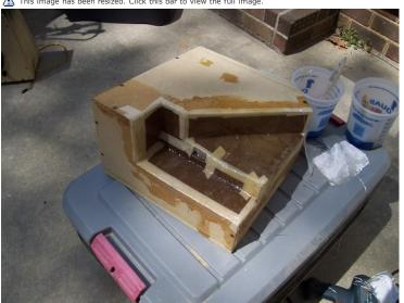
This part has been the biggest pain because it is around 90 degrees here today. Working time with the resin is 1-2 minutes, so I've mixed around 8 batches just to get 3 layers of cloth on this thing.
